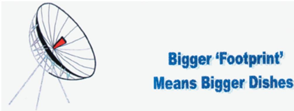
Cancom's rivals for the licence had chosen technology based on Ku-band satellite transponders, which operated on 14/12 Gigahertz and produced "spot beams" of concentrated power but limited coverage. Cancom elected to go with the broader "footprint" of 6/4 Gigahertz C-band, even though it required larger dishes. C-band had the added advantage of being available immediately. Ku-band would not be ready for at least eight months.
